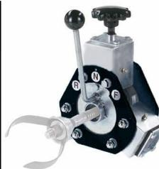
Superior for cable operation, this addition to your machine will make fighting stoppages easier than before. Grease fittings make maintenance quick and easy. Adjustable for any size cable.
